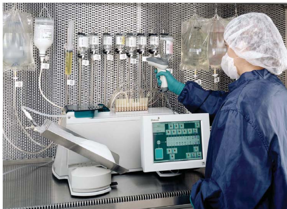
Baxa's Exacta-Mix 2400 is a 24-source compounder for both macro and micro ingredients.
