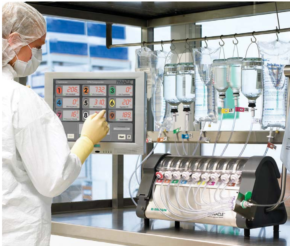
The Pinnacle TPN Management System from B. Braun is accurate within 2.5% for volumes above 20 mL.
