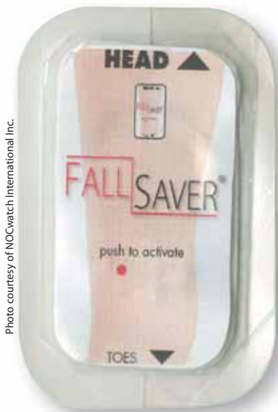
The FallSaver System from NOCwatch detects movement when a person's leg begins to bear weight.
