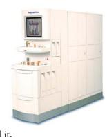
PharmASSIST ROBOTx is capable of incorporating dispensers from a customer's existing PharmASSIST SmartCabinet or Symphony+System, and is integrated with PharmASSIST Symphony workflow software. Enabling the throughput of up to 240 prescriptions an hour, the system labels, caps, and presents all filled vials to output queues from which operators can verify each prescription and then continue their prescription filling process.
